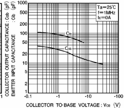
Fig.7 Collector output capacitance vs. collector-base voltage
