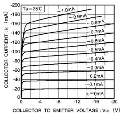
Fig.2 Grounded emitter output characteristics ( I )
