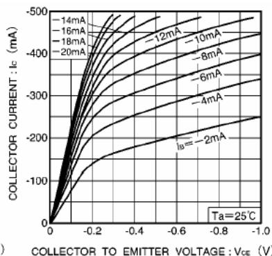
Fig.3 Grounded emitter output characteristics ( II )
